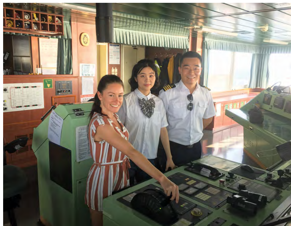
Cassandra poses on the bridge with the engine order telegraph, which is used to send speed instructions to the engine room.
